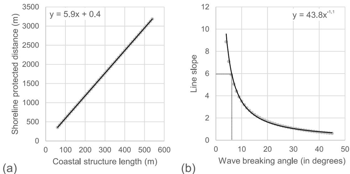
Figure 6.2. Correlation of: (a) coastal defence length and correspondent extension protected for  $6^\circ$  wave breaking angle; and (b) wave breaking angle and line slope of linear correlation between shoreline protected extension and coastal defence length.
